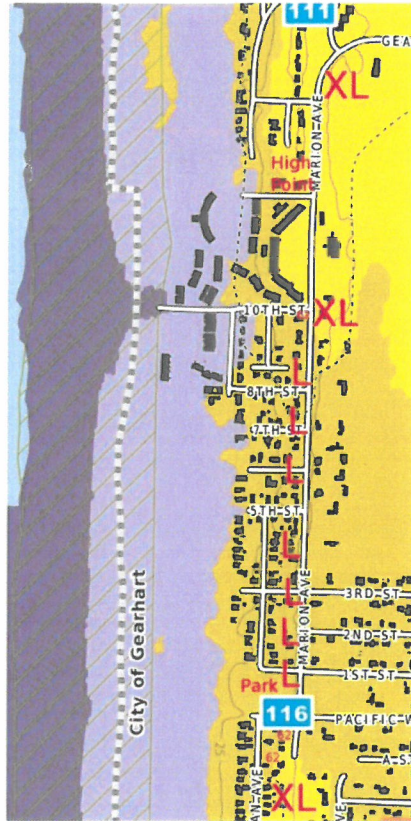
Figure 6: Gearhart tsunami inundation map showing L breaching Gearhart Park and crest of dune front at Ocean and Marion avenues, including the Gearhart Park site. LIDAR elevations of 62 feet are also noted within the L zone at the boundary with XL at Pacific Way and at 10th street, indicating the L1 scenario floods to 62 feet at the Park, which is 12 feet above the elevation of the proposed driveway of the Park station. Source: Priest et al. (2013). https://www.oregongeology.org/pubs/tim/p-TIM-Clat-08.htm LIDAR GIS at 54.200.239.5.
