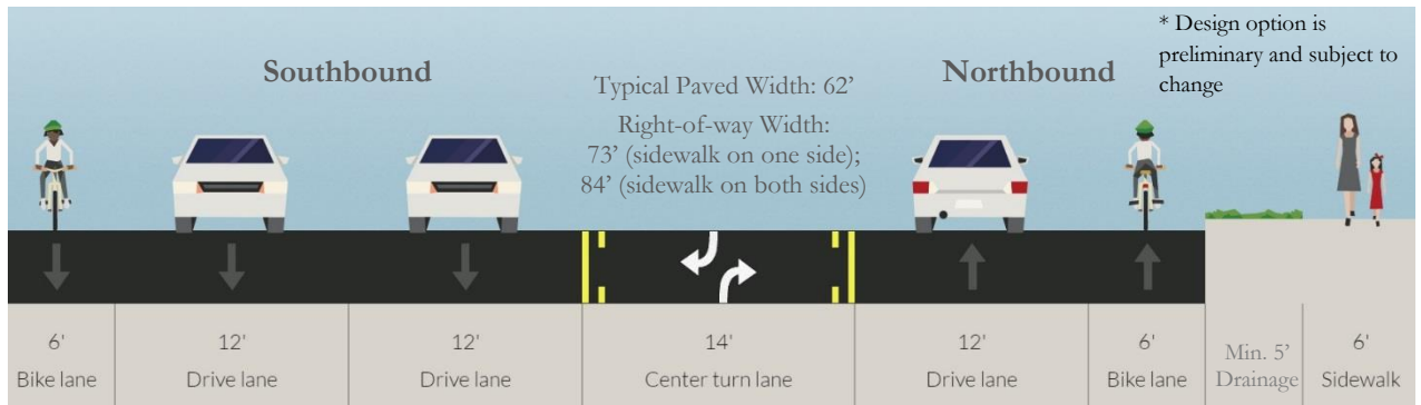
Option 2c: Reconfigure the street width of US 101 to include a center turn lane/median and bike lanes, and widen for a sidewalk
