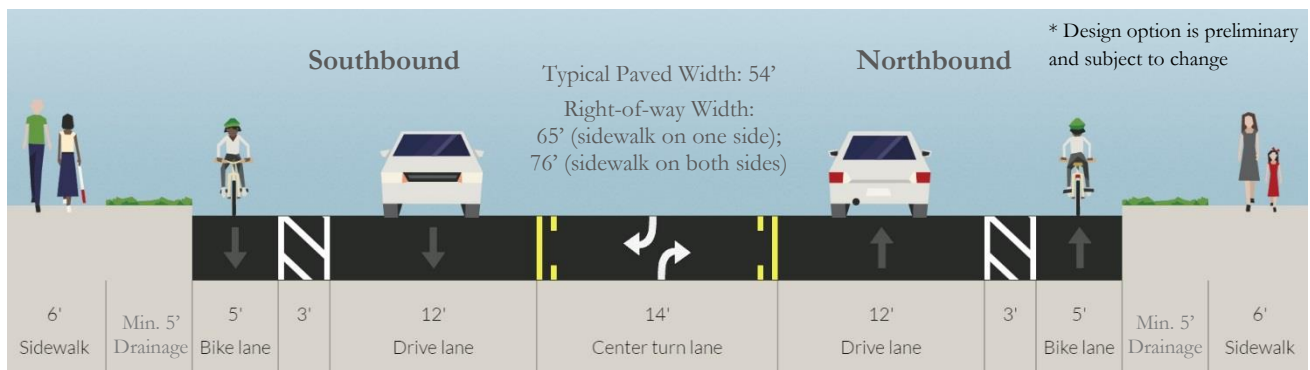
Option 3d: Reconfigure US 101 to three lanes and buffered bike lanes, and widen for sidewalks
