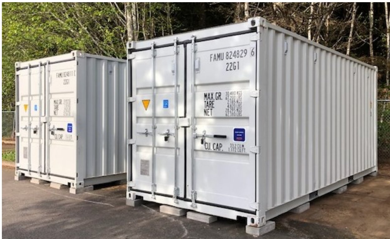
Figure 14: Two 20 ft Shipping Containers Elevated on 4x8x16" Solid Block Pavers for Airflow Photo courtesy of Susan Graves
