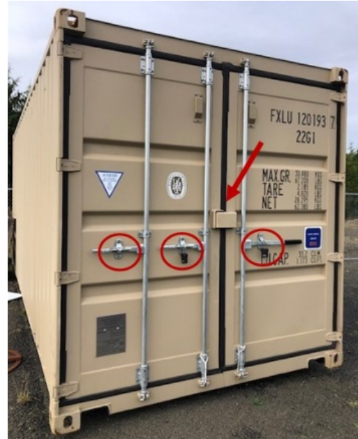
Figure 21: Padlock Configuration with Restricted-Access Lockbox in the Center Photo courtesy of Susan Graves
